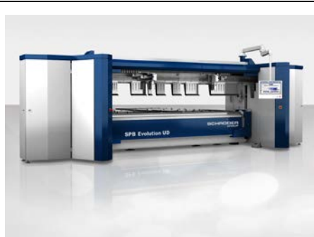
Folding machine SPB Evolution UD with fully automatic tool changer
