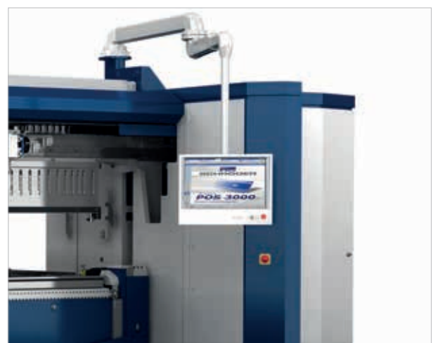
Software control POS 3000 of the folding machine SPB Evolution UD
