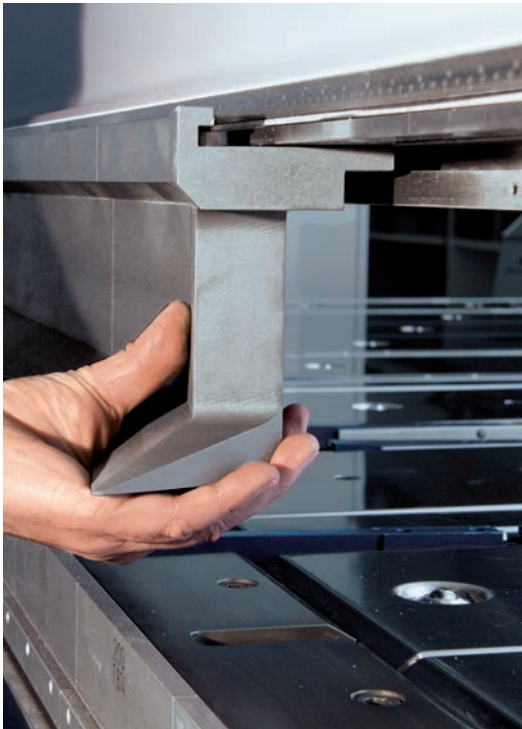
The optionally available hydraulic tool clamping device reduces set-up times.
