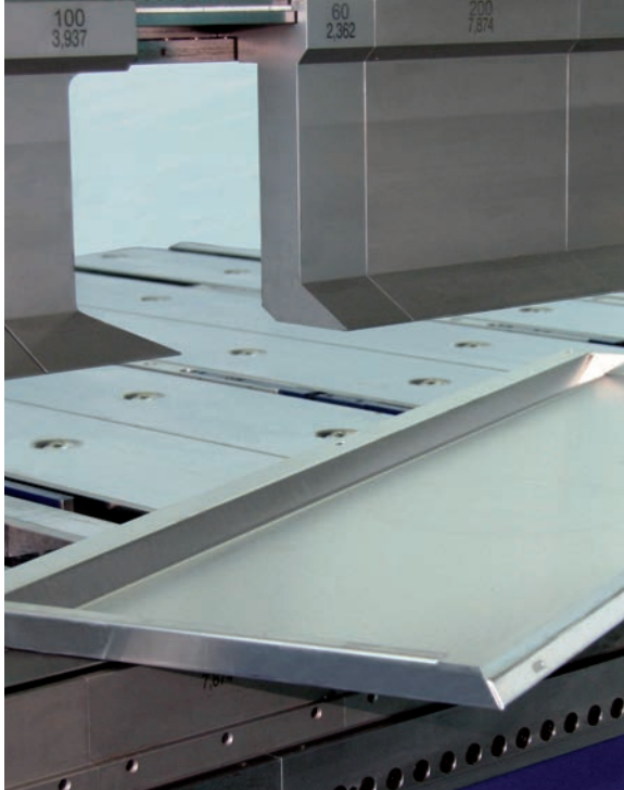
NEW: Clamping beam stroke of 500 mm for product heights of 250 mm.
