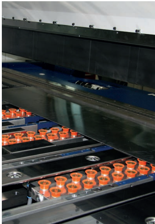
Suction plates in gauge table with 6 suction units, program-controlled incl. gauging against the folding beam (only for Up and Down).
