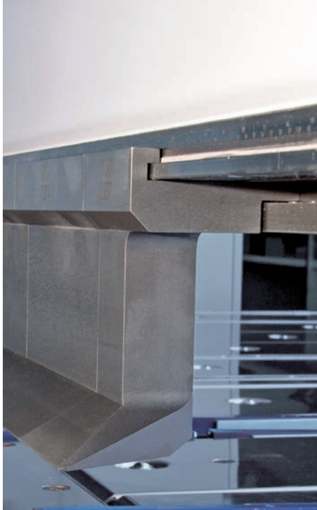
Segmented goat's foot blade, hydraulic tool clamping
