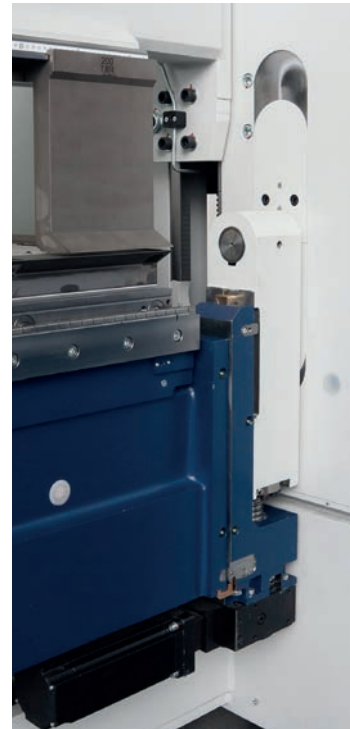
Folding beam lowering with servo drive and ball screws and servo controlled folding center adjustment.
