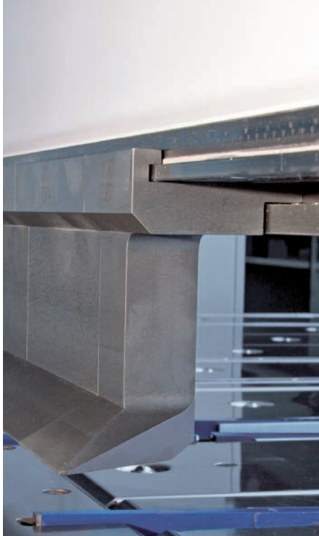
Segmented goat's foot blade, hydraulic tool clamping
