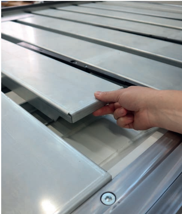
Standard: Removable support plates, retractable to 337 mm.
