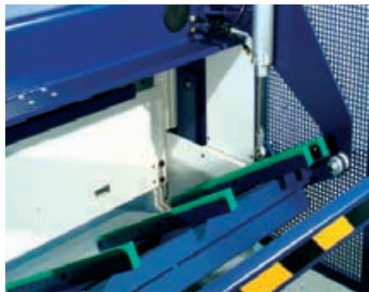
Sheet support to the front, pneumatically controlled, incl. sheet shute 750 mm or rather 1,000 mm
