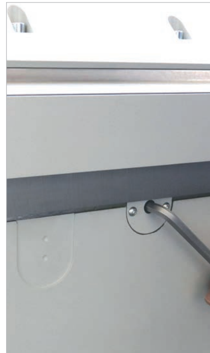
Crowning device for folding beam: manual central crowning device (not in combination with cranked folding blades).
