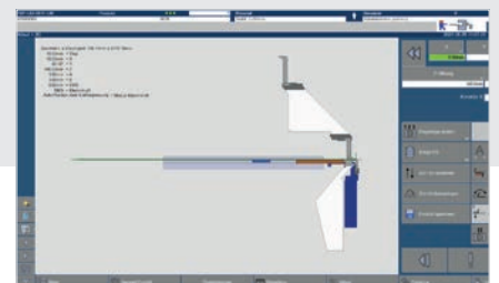
Above: Standard bending programs are available in the product selection menu. Below: The software shows the processing steps beforehand.
