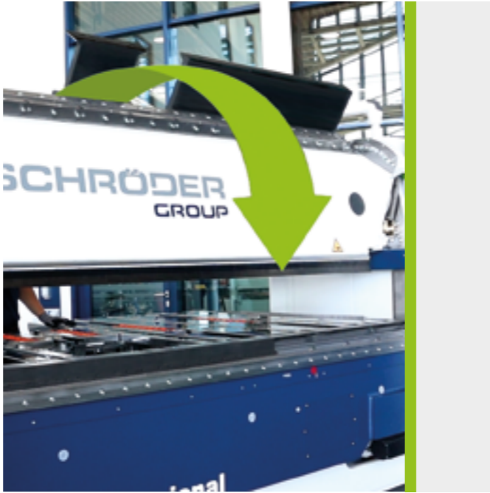
The rotating clamping beam offers a second set of tools and an alternative machine geometry. (New: Clamping beam directly driven with servo motors)
