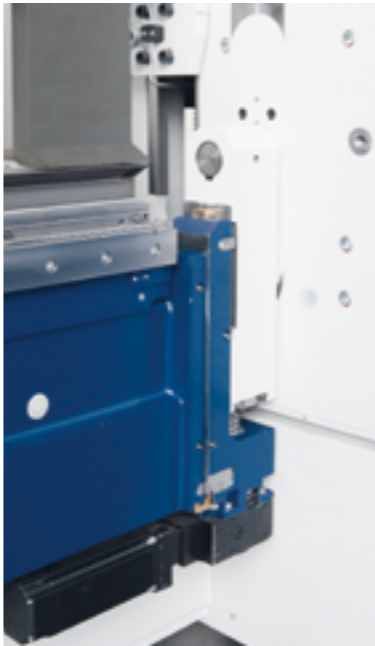
Folding beam lowering with servo drive and recirculating ball screws
