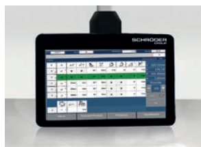
Classic Bend control on swivelling arm: a modern, alphanumeric control system
