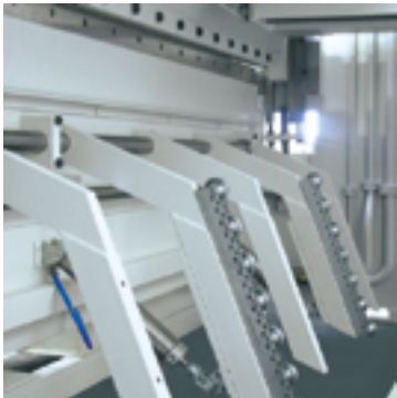
Pneumatically controlled sheet support
