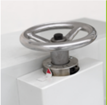
Manual blade gap adjustment
