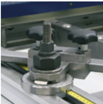
Angle gauge adjustable 0-360° according to scale
