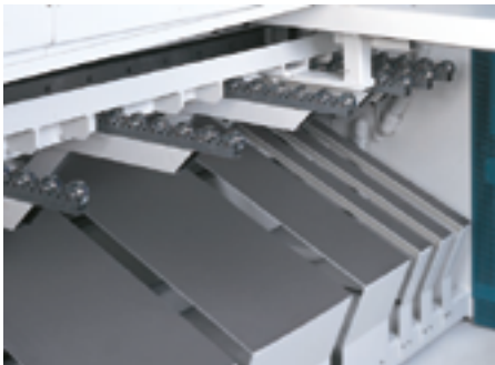
Pneumatically controlled sheet support incl. sheet shute in active mode.
