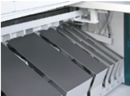
Pneumatically controlled sheet support incl. sheet shute in non-active mode.
