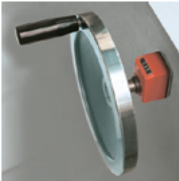
Manual blade gap adjustment
