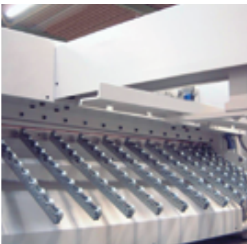
Pneumatically controlled sheet support with ball castors.
