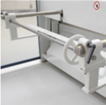
Manual back gauge, adjustment range 10 - 600 mm
