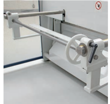
Manual back gauge, adjustment range 10 - 600 mm
