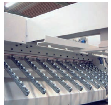
Pneumatically controlled sheet support with ball castors.
