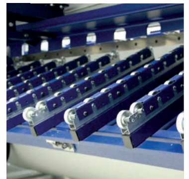
Sheet support, pneumatically controlled
