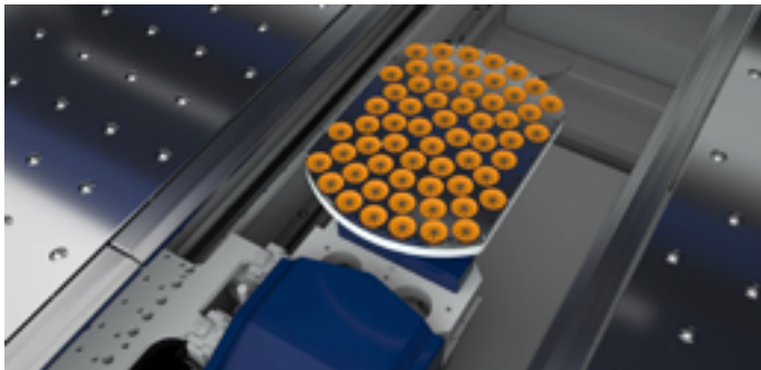
Option: The rotary plate gauge system is a fully automatic advanced handling system "AHS" with a camera system for measuring the sheet contour.
