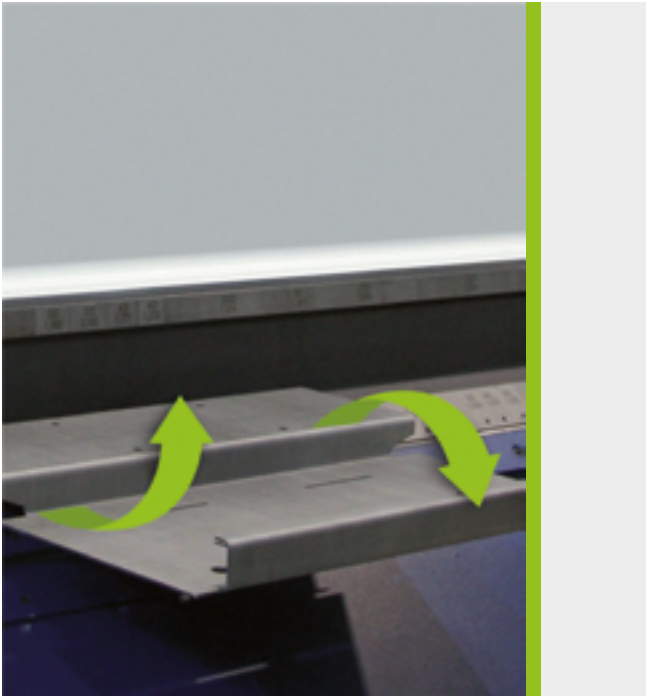
The Up-and-Down folding beam allows counterbends in one working step.
