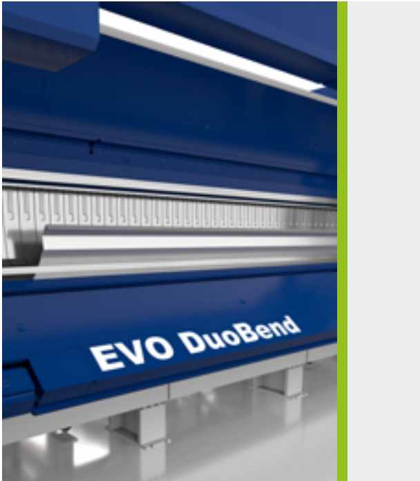
Thanks to the two folding beams the machine is able to bend a large number of counterfolds one after the other. The prime example of such workpieces is a customer-specific trapezoidal sheet.
