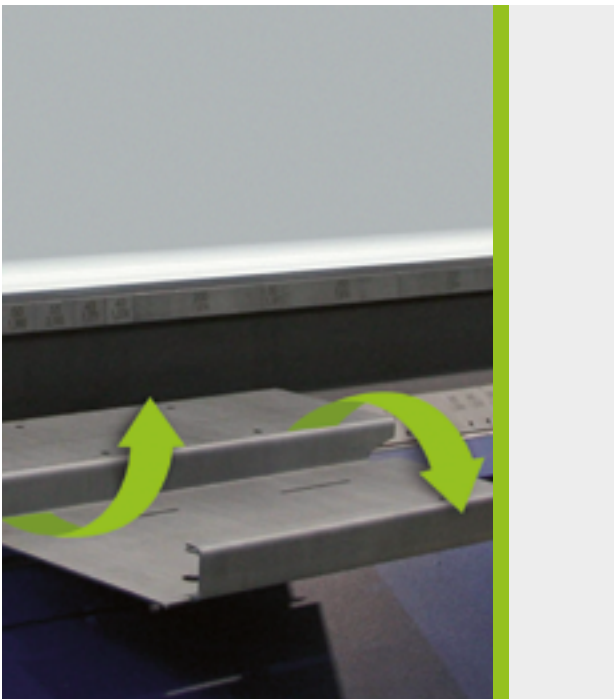
Up-and-Down function: counter folds without turning the sheet
