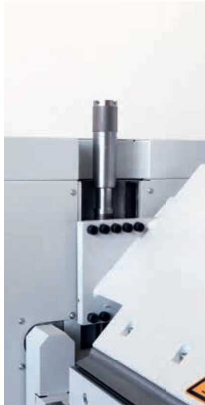
Clamping pressure adjustment of the clamping beam
