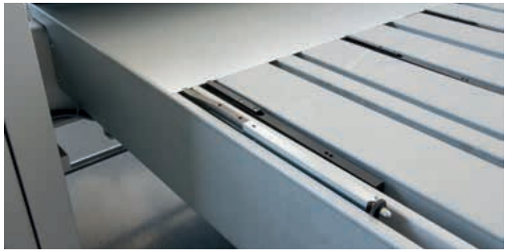
Picture above: Sheet support table with steel balls Picture below: adjustable back gauge fingers for conical bending
