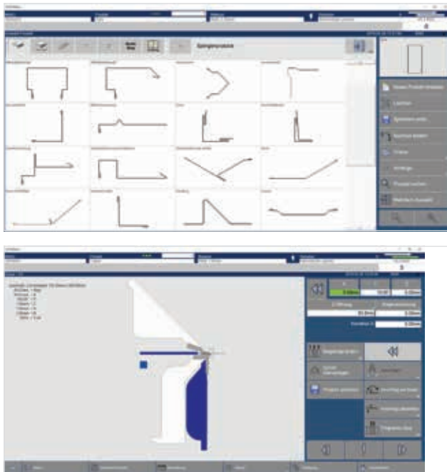
Graphic control POS 2000 Professional: the result always visible – from the first bending steps up to simulation
