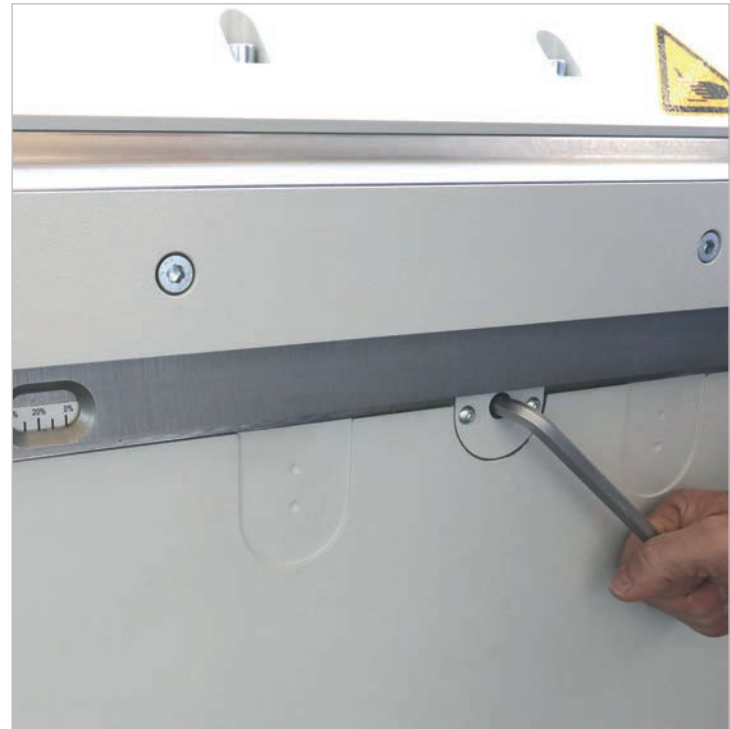
Crowning device for folding beam: manual central crowning device (not in combination with cranked folding blades)
