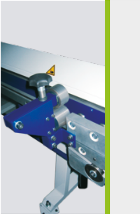
One function of the cutting- and flattening device is to close folding edges
