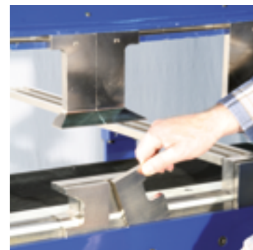
Patented quick clamping device with eccentric for clamping- and folding beam
