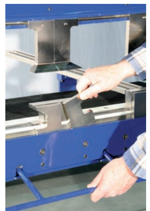
Patented eccentric fast clamping for the clamping and folding beam
