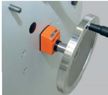
Standard: Digital Siko-display for manual bottom roll adjustment needed for sheet thickness adjustment, optionally also available motorized.
