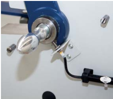
Option: with interchangeable roll the top roll diameter gets automatically detected by an initiator.
