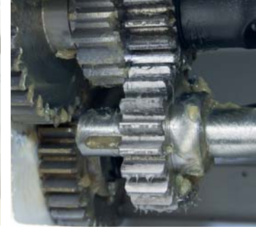
Change gear top roll for interchangeable roll
