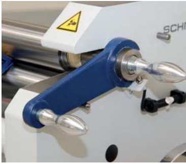
Standard: Pivot bearing for opening the top roll
