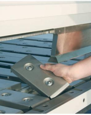
Back gauge: optional with conical bending function.
