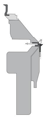
Cross section tool: Tinsmith blade 20°, R 1/1.5, directly screwed, cranked folding blade
