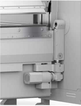
To suit your typical sheet metal formats, we offer various gauge systems with pneumatically lowerable gauge fingers and ball rollers for easy and gentle movement of the workpiece.
