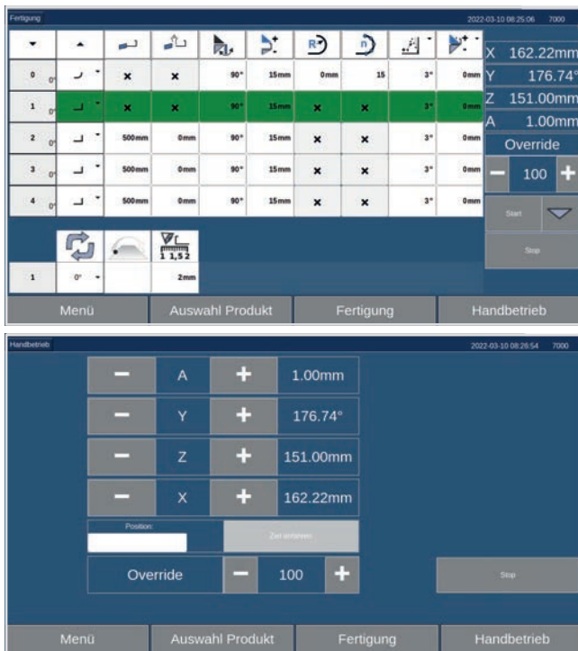
Simple symbols and alphanumeric data describes the bending program.
