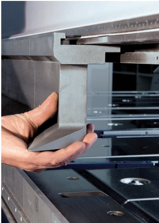
The optionally available hydraulic tool clamping device for the clamping beam reduces set-up times.
