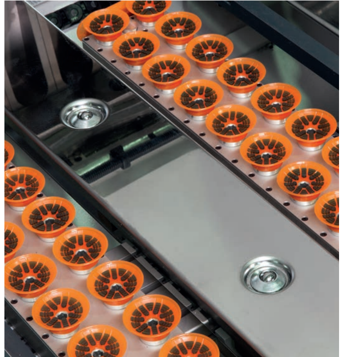
Suction plates in the back gauge table, controlled via POS 3000.
